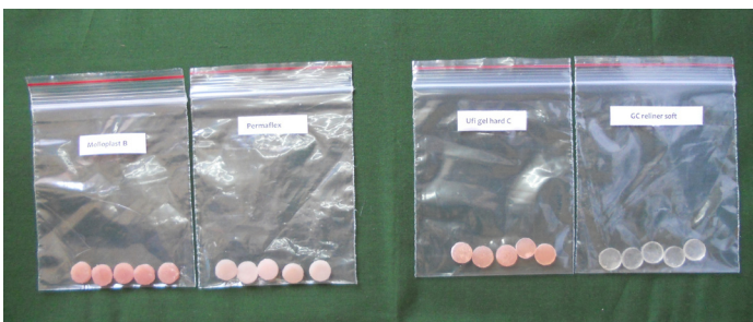
[Table/Fig-3]: Test discs of Permaflex, Molloplast B, Ufi gel hard and GC soft liner with smooth surface on one side and rough on the other.
