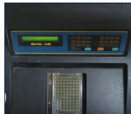
[Table/Fig-1]: Wells coated with test materials. [Table/Fig-2]: Transfer of brain heart infusion broth to the microtiter wells. [Table/Fig-3]: Elisa Reader (Stat Fax 2100) (Awareness Technology).
