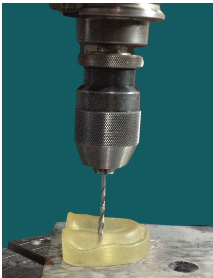
[Table/Fig-2]: Milling of epoxy resin casts.
