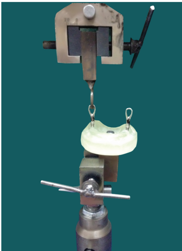
[Table/Fig-6]: Testing of cemented crowns on universal testing machine
