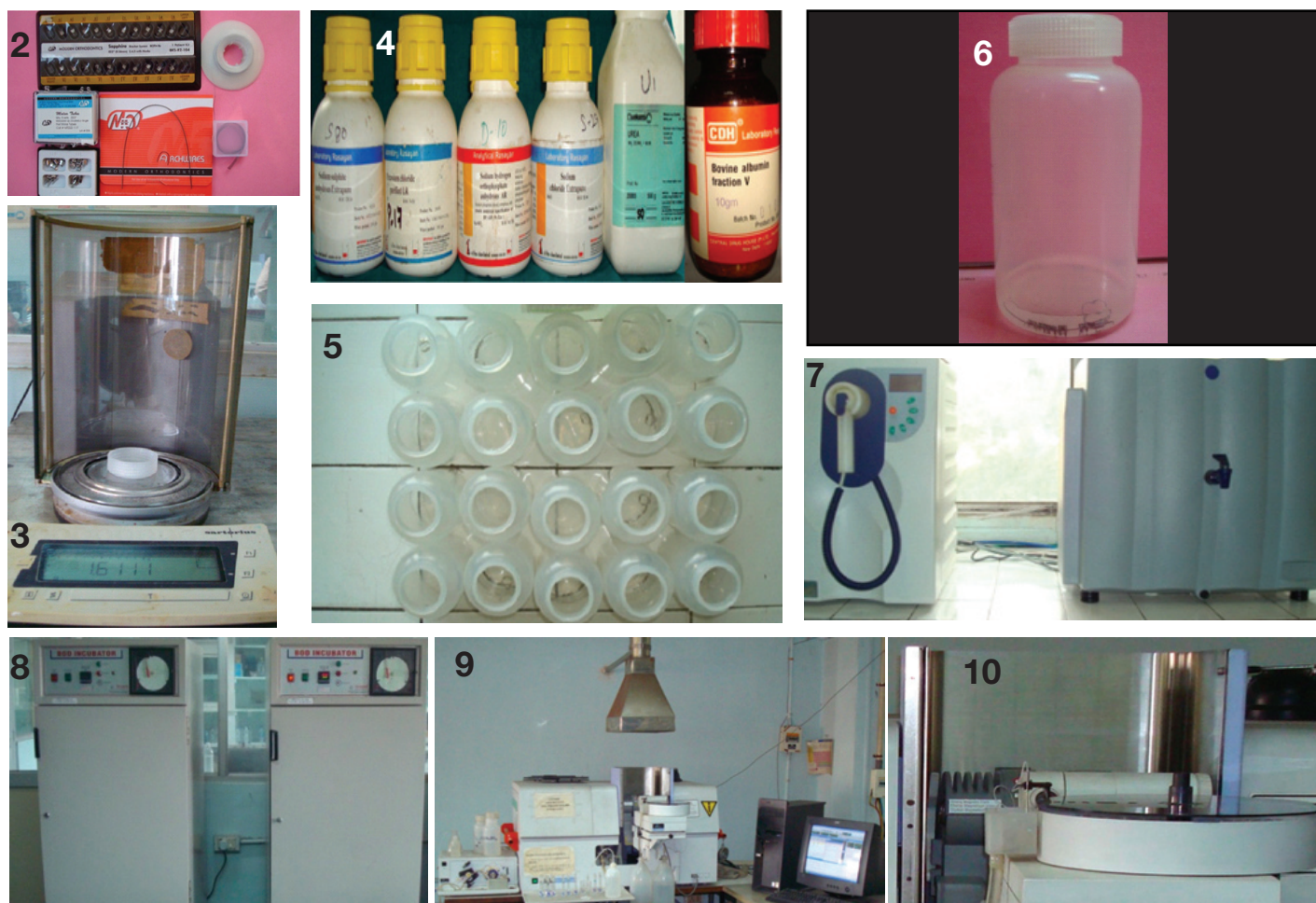
[Table/Fig-2]: Orthodontic materials (Modern orthodontics, Ludhiana). [Table/Fig-3]: Electronic weighing machine. [Table/Fig-4]: Constituents of artificial saliva. [Table/Fig-5]: Twenty Samples in the polyethylene bottles. [Table/Fig-6]: Appliance dipped in the artificial saliva. [Table/Fig-7]: Three stage water purification system. [Table/Fig-8]: Incubator. [Table/Fig-9]: Atomic absorption spectrophotometer. [Table/Fig-10]: Close-up view of auto sampler unit with graphite furnace
