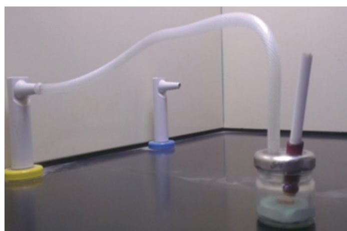
[Table/Fig-3]: Smoking machine assembly fastened in vacuum pump machine
