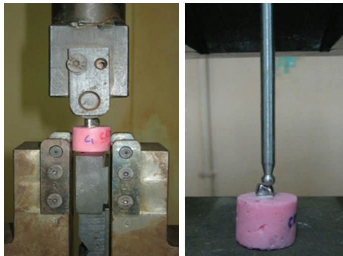
[Table/Fig-2]: Cyclic loading in artificial chewing simulator [Table/Fig-3]: Static loading in universal testing machine
