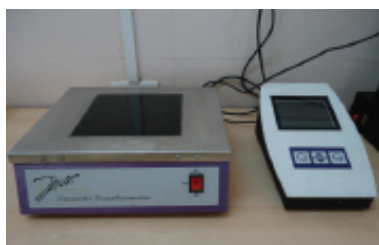
[Table/Fig-5]: UV transilluminator with Gel documentation
