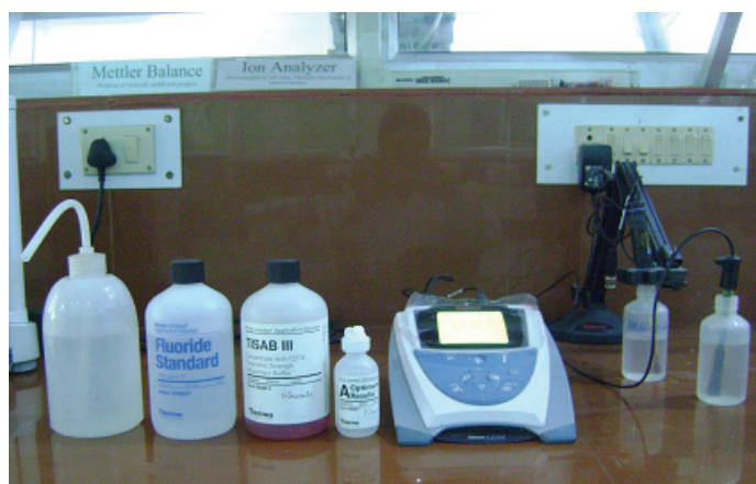
[Table/Fig-1]: Fluoride ion selective electrode (Orion-9609BNWP) coupled to an ion analyser used for measurement of Fluoride ion concentration
