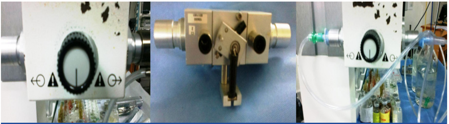
[Table/Fig-2]: Faulty switch over knob of anaesthesia machine and demonstration of bi directional flow
