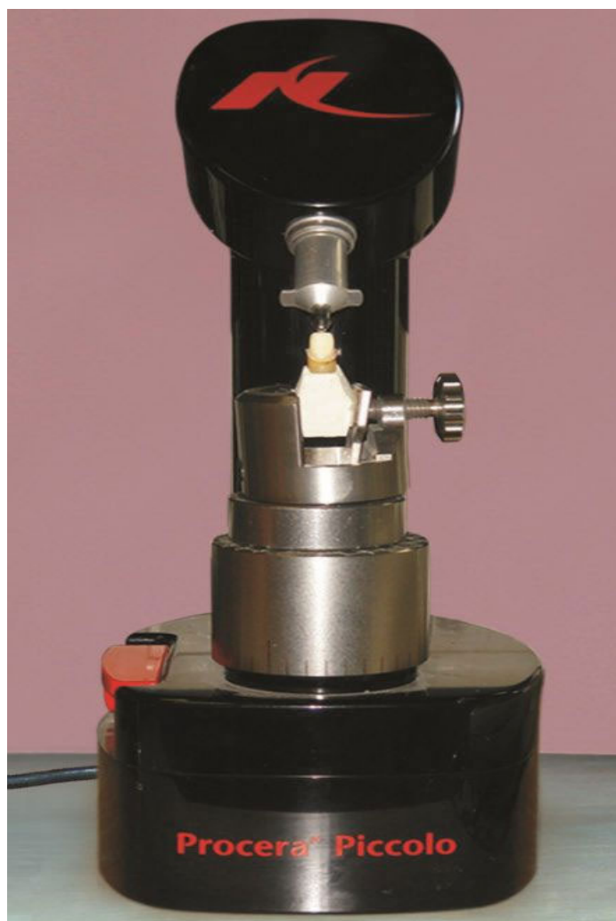
[Table/Fig-3]: Scanning of the prepared tooth With Procera scanner
