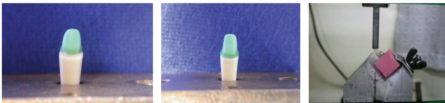
[Table/Fig-4]: Wax pattern with extension of labial margin 1mm short of gingivoaxial line angle of finish line (Group B) [Table/Fig-5]: Wax pattern with 0.4mm wide facial collar margin (Group C) [Table/Fig-6]: Load application on one of the specimen
