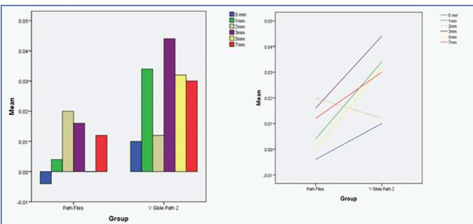
[Table/Fig-10]: (A) Bar graph (B) Line graph: showing the comparison between the two groups indicating canal transportation was statistically significant at all the intervals except at 1mm between the instruments
