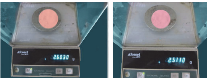
[Table/Fig-4]: Samples weighed before testing for sorption & solubility
