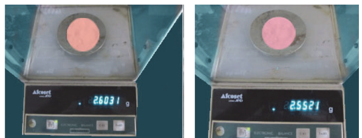
[Table/Fig-8]: Samples weighed again to check water sorption by the material
