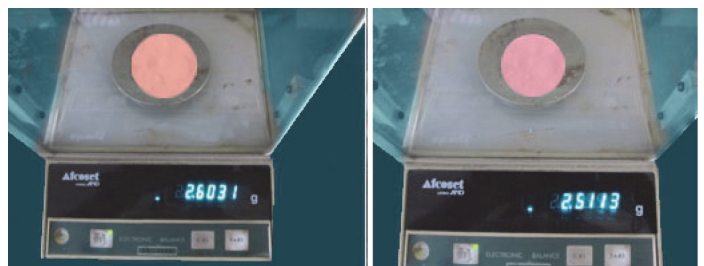
[Table/Fig-6]: Samples weighed again to check till weight loss did not differ more than 0.5 mg
