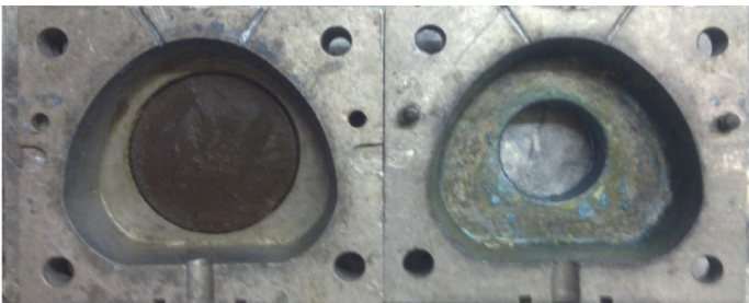
[Table/Fig-2]: Aluminium denture flasks meant for injection moulding procedure
