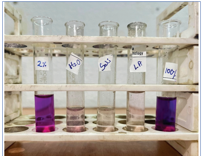
[Table/Fig-3]: Test tubes with formalin solutions (2% and 100%) and controls (saline, distilled water, local anaesthetic). Only formalin solutions turned purple, with colour intensity increasing with concentration; controls remained colourless.
