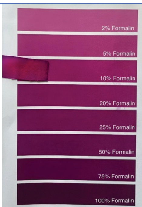
[Table/Fig-6]: Filter strips produced consistent colour changes that closely matched the established colour palette.
