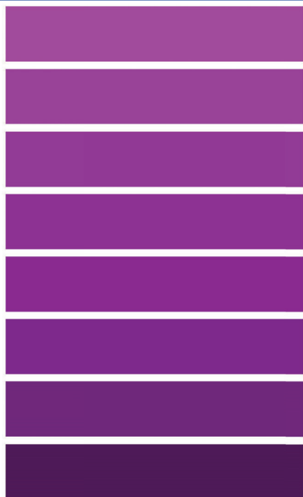
[Table/Fig-4]: Colour palette illustrating the gradient from light to dark purple with increasing formalin concentrations (2% to 100%) after adding Schiff's reagent.
