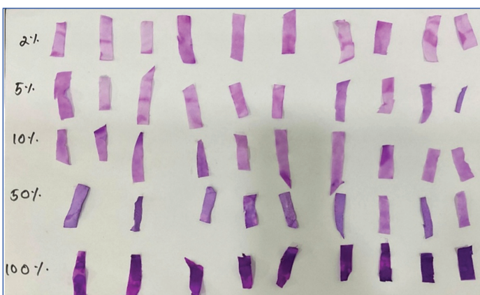
[Table/Fig-5]: Filter paper strips dipped into the formalin solutions shows progressive intensification of colour from the 2% to the 100% formalin concentrations.
