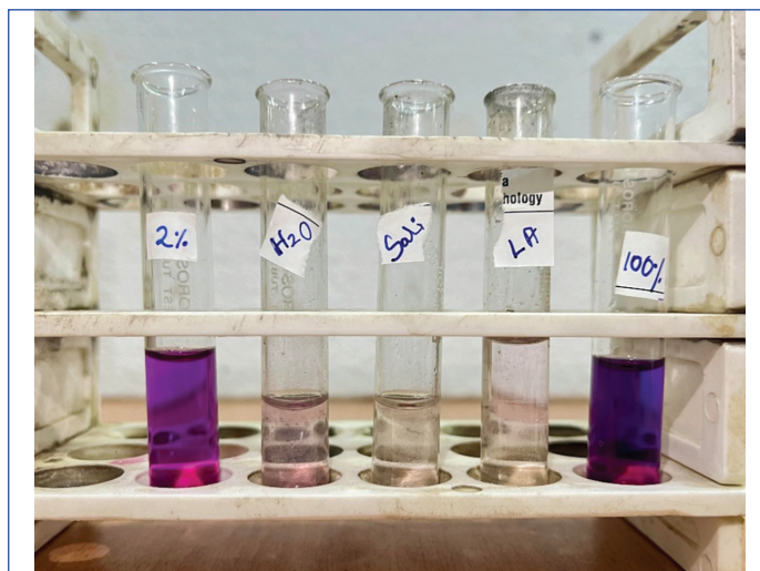
[Table/Fig-3]: Test tubes with formalin solutions (2% and 100%) and controls (saline, distilled water, local anaesthetic). Only formalin solutions turned purple, with colour intensity increasing with concentration; controls remained colourless.
