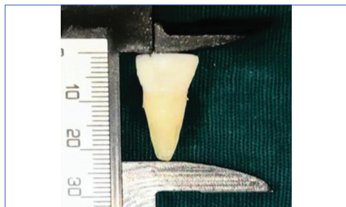
[Table/Fig-1]: Sample has been cut coronally to maintain the equal length of 22 mm.
