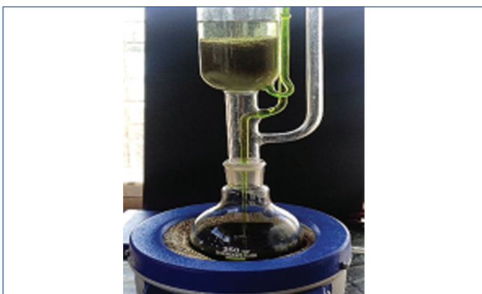
[Table/Fig-1]: Soxhlet apparatus used for the extraction of Nyctanthes arbor-tristis leaf samples with different solvents.
