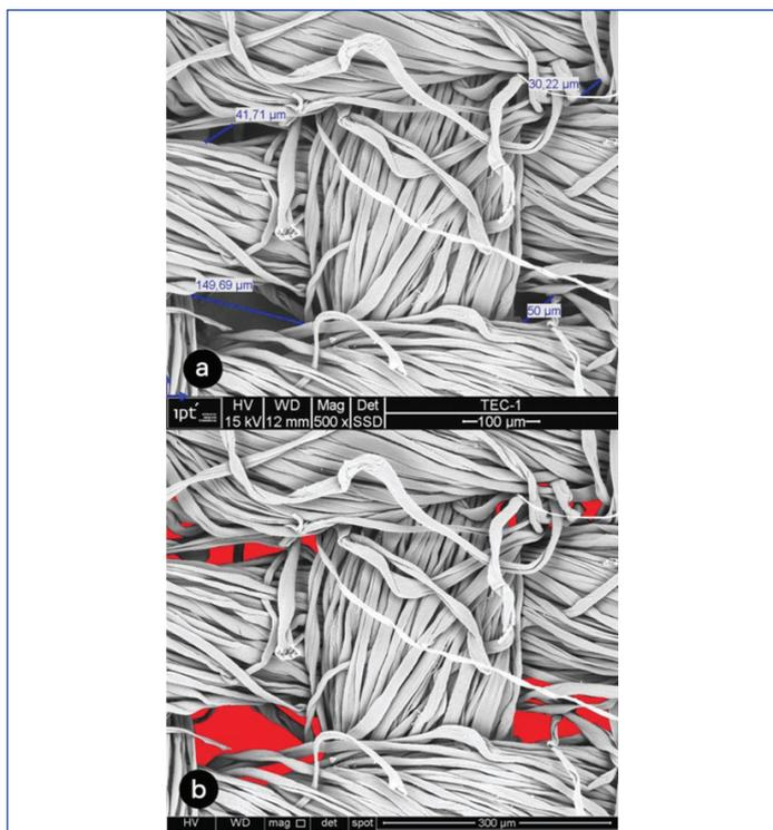
**[Table/Fig-2]:** (500 X) Photomicrographs of cloth mask. a) visualisation of distance among threads; b) gap spaces (red mark).
