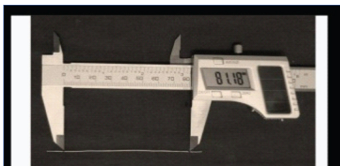
[Table/Fig-2]: Measurement of marked length of brass wire using a digital vernier caliper.
