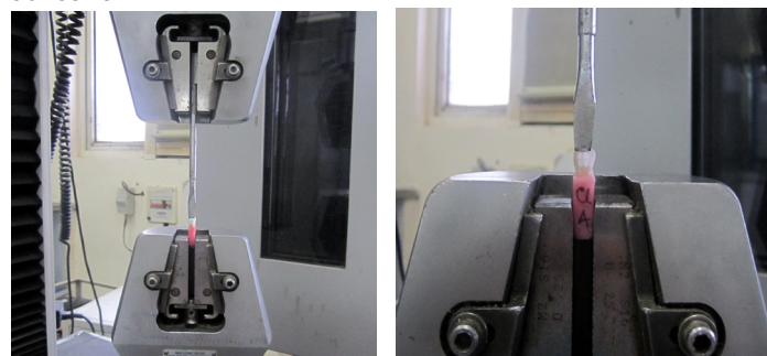
[Table/Fig-3]: Universal testing machine with mounted specimen.
