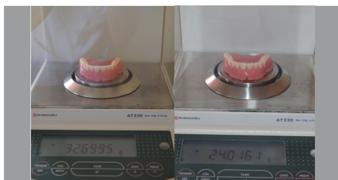
[Table/Fig-10]: Difference in the weight of conventional and hollow maxillary complete denture.
