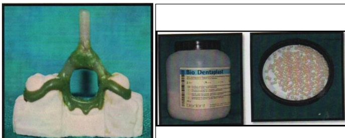
[Table/Fig-1]: Wax pattern adapted on refractory cast. [Table/Fig-2]: Acetal resin granules.
