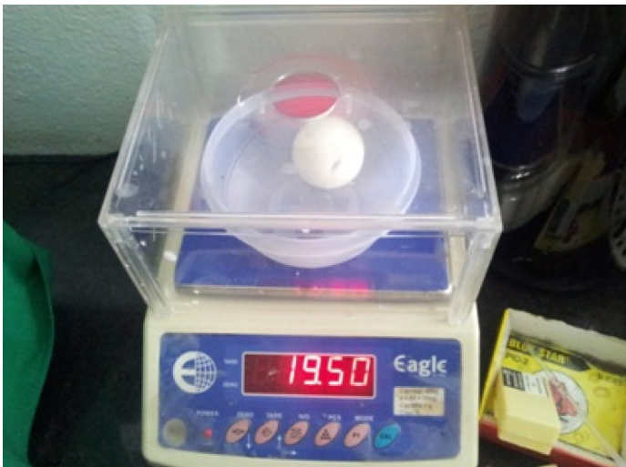
[Table/Fig-9]: Measuring each sample weight by electronic weighing machine.
