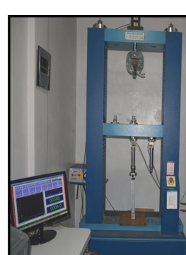
[Table/Fig-3]: Metal Jigs. [Table/Fig-4]: Metal jigs with wire and module dipped in artificial saliva. [Table/Fig-5]: Universal testing machine. [Table/Fig-6]: Testing jig mounted on universal testing machine.
