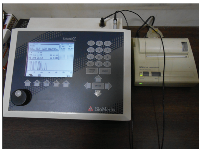
[Table/Fig-1]: Ultrasound machine 'Biometric A-Scan' that was used for measuring the palatal gingival thickness
