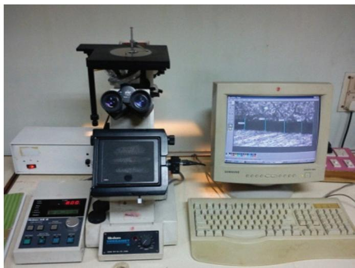
[Table/Fig-3]: Stereomicroscope (Versamet 3., Union Opt. Japan. With Clemex Image analyzing system)
