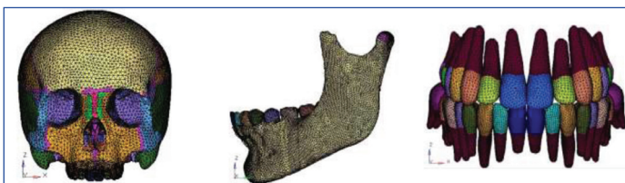
[Table/Fig-4]: Finite element mesh model of human skull and teeth.
